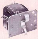
Scope power transformer with board for rectifiers. Primary 115 V., 400 cycles to two 14 KV filament windings, one 6.3 V. low capacity filament winding, 4.5 KV and 1.75 KV high voltage windings. 25 KV hipot when in oil; 21/8 x 31/2 x 25/8", 11/4 lbs.
