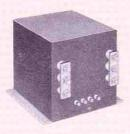
High current filament transformer. Primary 140/156 V., 47/63 cycles to 1.8 V.-1070 A. Current limiting through separate primary reactor, MIL-T-27A; 10 x 10 x 11½", 150 lbs.
