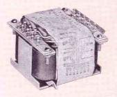
230° C. power transformer. Primary 115 V., 3 phase, 300/420 cycles to 200 V. and 20 V. secondaries, 525 V.A. 230° C. operating; 23/4 x 3 x 2", 1.8 lbs.
