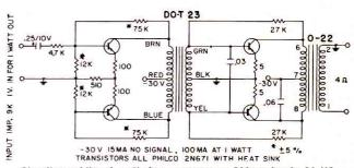
Circuit providing 1 watt, frequency range 200 cycles to 20 KC
