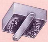
Instrument reference transformer. Input 50 V. 400 cycles. Three 5 V.-025A. Outputs to .05% accuracy. Saturation characteristics and DCR balance to 3%. MIL-T-27A; 1½ x 1¾ x ¾, 2 oz.
