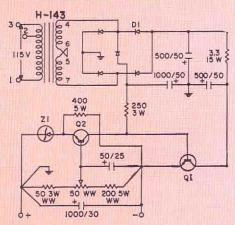
DI (5) .75A 100 PIV ZI 6.8V ZENER (1.5M 6.8Z) QI DELCO 2N441 (SINK 7270725) Q2 RCA 2N301 (HEAT SINK)
