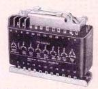
Molded Power Transformer 3 Phase. Input 200V, 380-420 cps. Electrostatic Shield, 8 output windings. 26 terminals. MIL-T-27A, Grade 2 Class S. Max. Alt. 50K Ft. Size 6 x 2½ x 5", 8 lbs.
