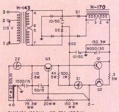
D2 .75A , 100 P.I.V. DI (4) 1.5A . 100 P.I.V. ZI 12V ZENER (IN1513) Z2 3.9V ZENER (IN1507) QI PHILCO 2N671 (HEAT SINK) Q2 DELCO 2N441 (SINK 7270725) Q3 TEXAS 2NI377
