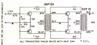
Circuit providing 140 MW, frequency range 300 cycles to 20 KC
