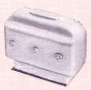
High temperature plate transformer. Primary 208 V., 3 phase 380/1000 cycles to 5100 V./leg, 1400 V. A. 200° C. MIL-T-27A; 6 x 3 x 4½", 6 lbs.
