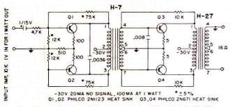
Circuit providing 1 watt, frequency range 100 cycles to 20 KC
